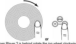
When Player 2 is behind rotate the jog wheel clockwise or press to bend pitch faster
